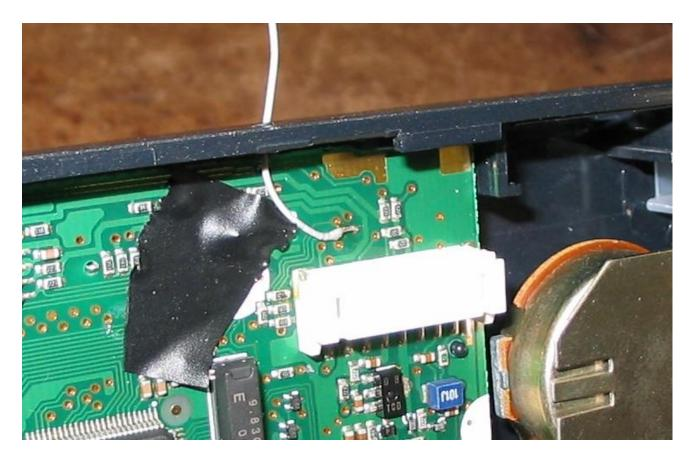
Disregard the piece of electric tape. I was initially going to make a strain relief. I decided to use a small knot instead.
