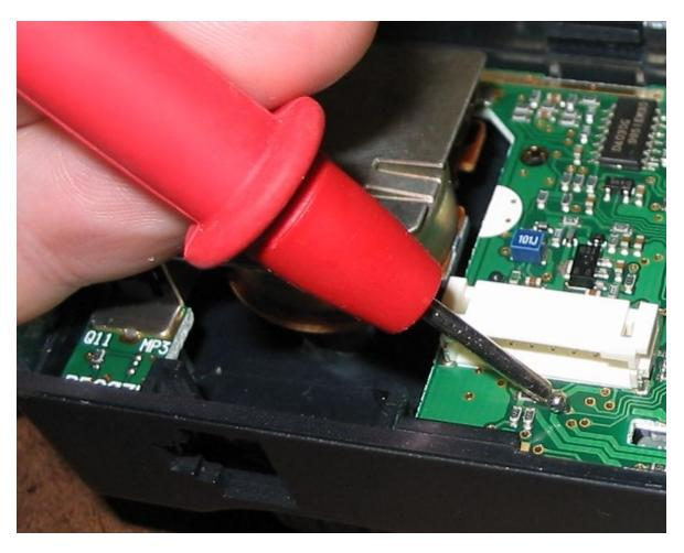
Solder a thin insulated wire to this point. I would recommend drilling a tiny hole for the wire, but I am sure you could also find a creative way to exit the radio head.
